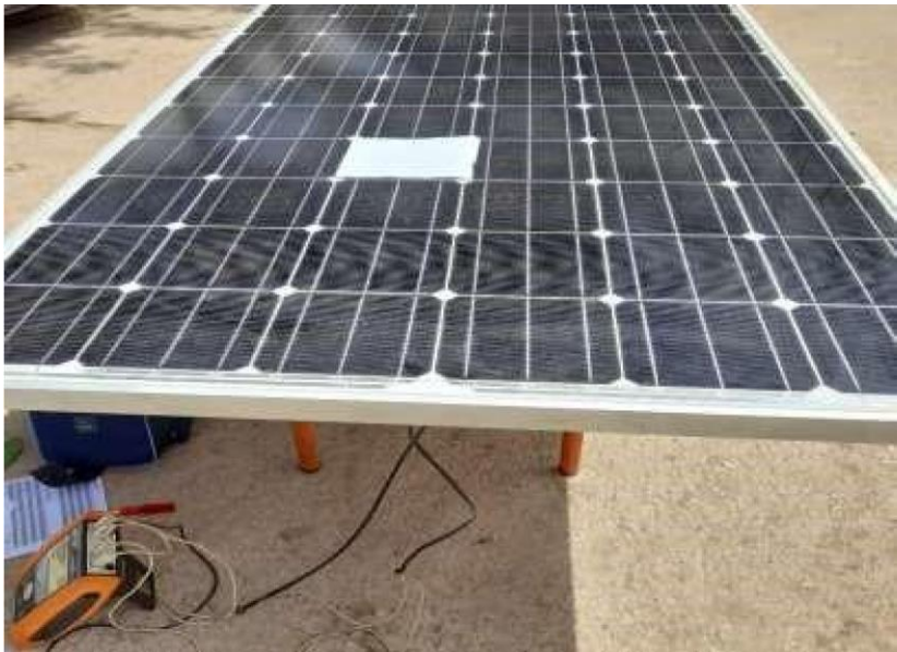
Figure 1. Mono module under test in partial shade. Source: results of my work Table 1. Technical characteristics of monocrystallin and polycristallin panel in STC.
