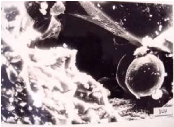
Figure 4 (10μ). Scanning electron microscope (S.E.M.), photomicrograph showing rough surface texture with platy crystalline particles whitish coating on atmospheric exposure with whitish small secondary slag blebs.
