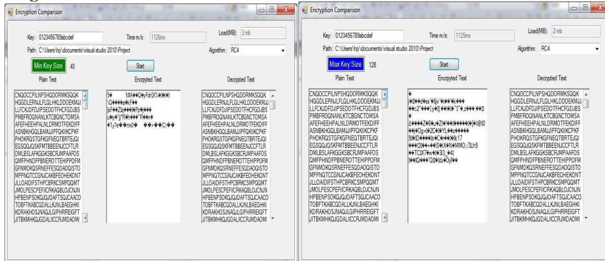
Figure 2: GUI Simulation of RC4 algorithm minimum and maximum key size encrypt/decrypt testing
