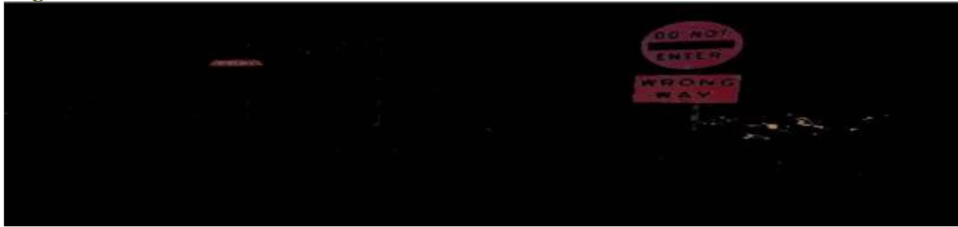
Figure 5. Color segmentation for red traffic signs.
