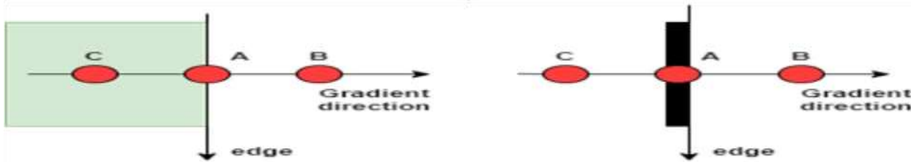
Figure 6. Suppression of non-maximum edges in Sobel edge detection.
