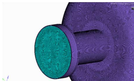
Figure 4: Model of the fluid meshing
