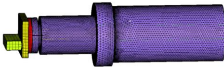
Figure 6: The whole model meshing
