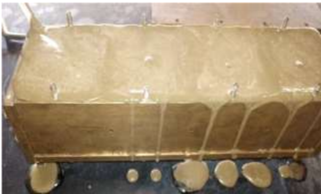
Figure 9. Cement slurry poured into a brass mold vessel Figure 10. The brass mold in the pressure vessel
