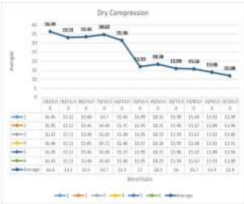
Figure 14: Variation of Dry Compressive Strength with Various blends of Itakpe/Agbaja Iron Ore Pellets Indurating Compressive Strength Test @ 1200°C (N/P)
