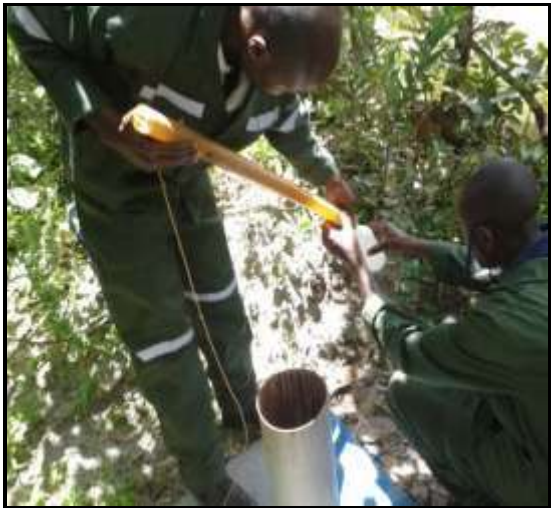
Figure7: Water sampling – Borehole JM8 DISCUSSIONS
