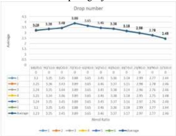
Figure 11: variation of Drop Number with various blends of Itakpe and Agbaja Iron Ore Pellets
