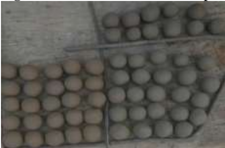
Figure 10: Shows how some resultant pellets for both Itakpe and Agbaja iron ores as been dried in the normal atmospheric which is known as green pellets
